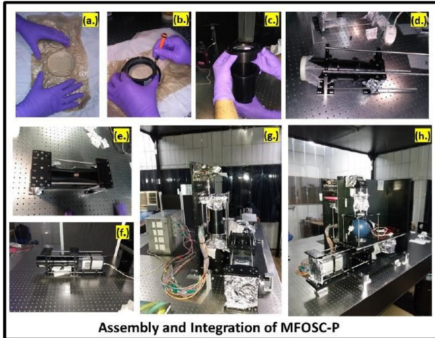
Figure 1: Panels (a.), (b.) & (c.) show the development of MFOSC-P lens barrels. Panels (d.), (e.) and (f.) show the completed lens barrels and their cage-rod assemblies. Panels (g.) and (h.) show the assembled MFOSC-P instrument in the laboratory.
